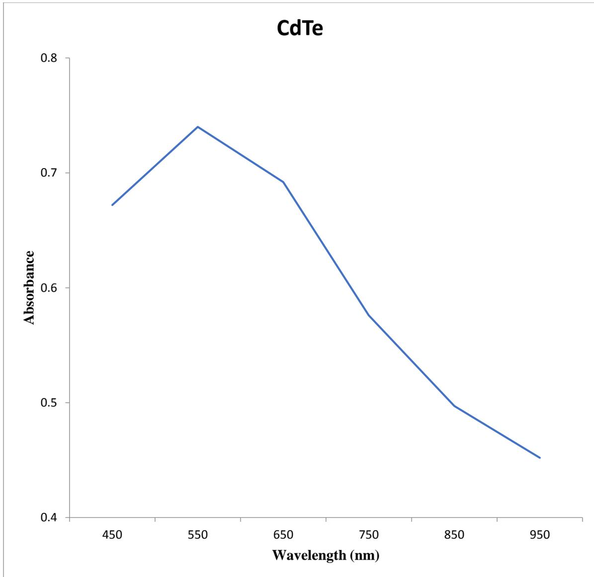
Figure 1b: Absorbance against wavelength of the Annealed CdTe thin film
