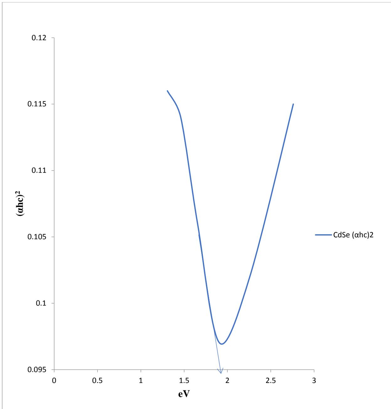
Figure 2: Graph of  $(\alpha hc)^2$  plotted as a function of the photon energy (eV) for CdSe Thin Film
