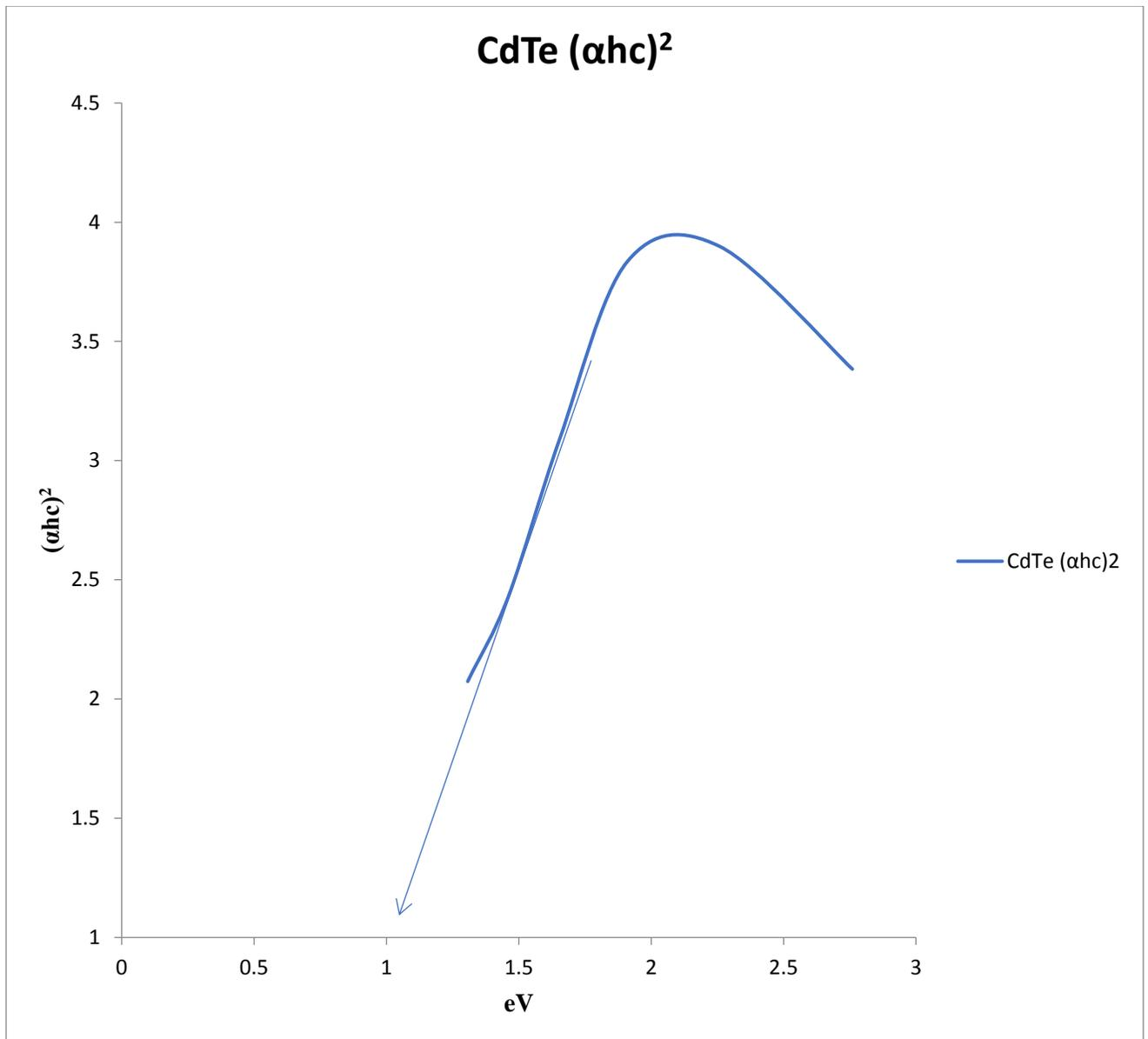
Figure 3: Graph of  $(\alpha hc)^2$  plotted as a function of the photon energy (eV) for CdTe Thin Film
