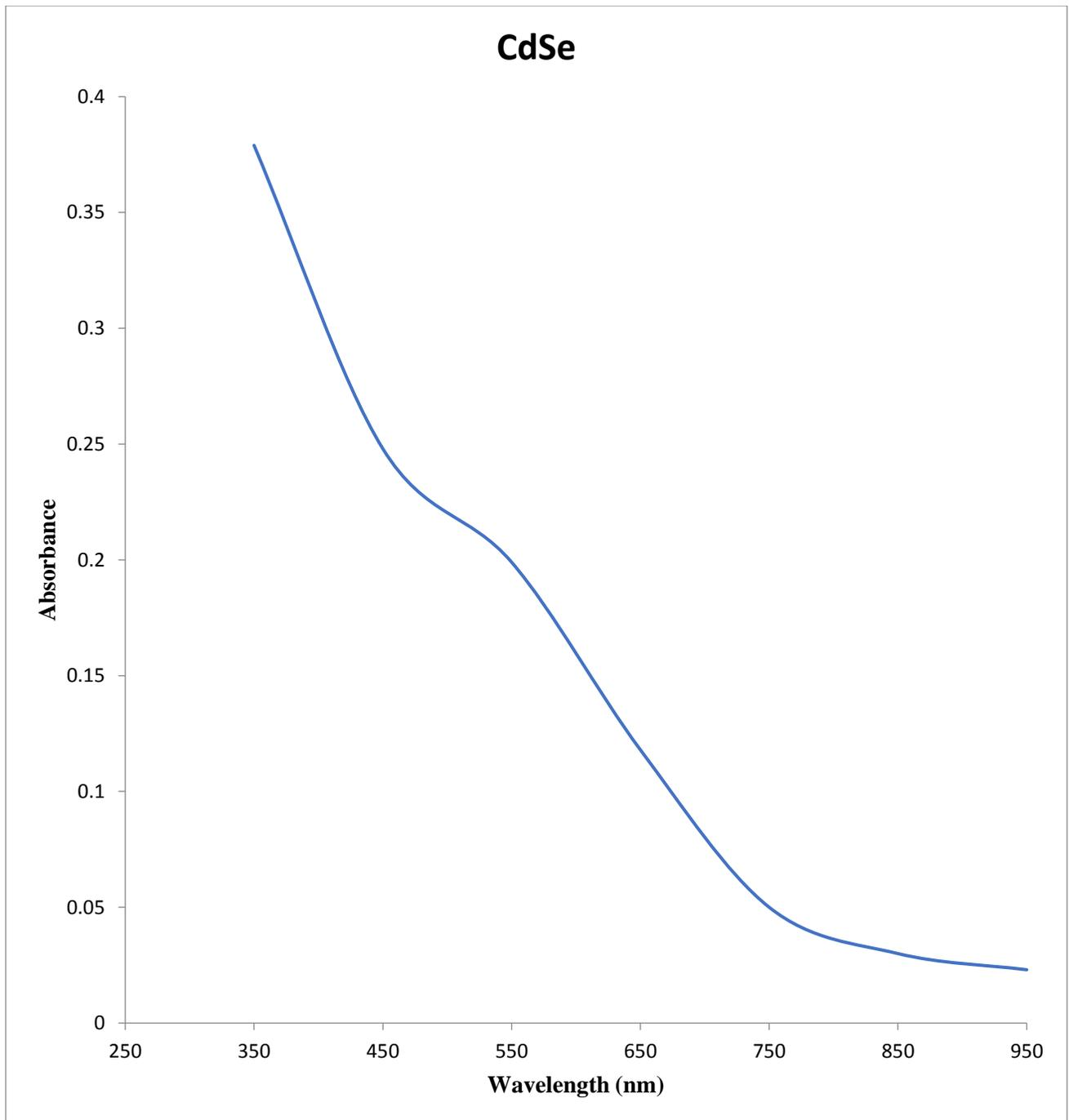
Figure 1a: Absorbance against wavelength of the Annealed CdSe thin film
